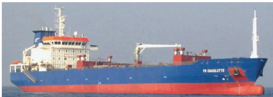
*FS Charlotte* can carry alternate cargoes of liquid sulphur and bitumen
